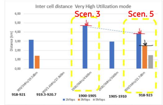
Again the case of 1900MHz at max DL power (43dBm) offers the biggest inter-cell distance solution for 1Mbit/s requirement while the 900/5MHz/21.7dBm offers a solution in the range of up to 2.6Km for 3Mbps.
