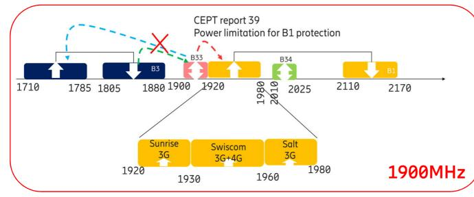
Blocking and co-existence impact to adjacent spectrum blocks determine the guard bands and maximum allowed DL power that can be transmitted.
